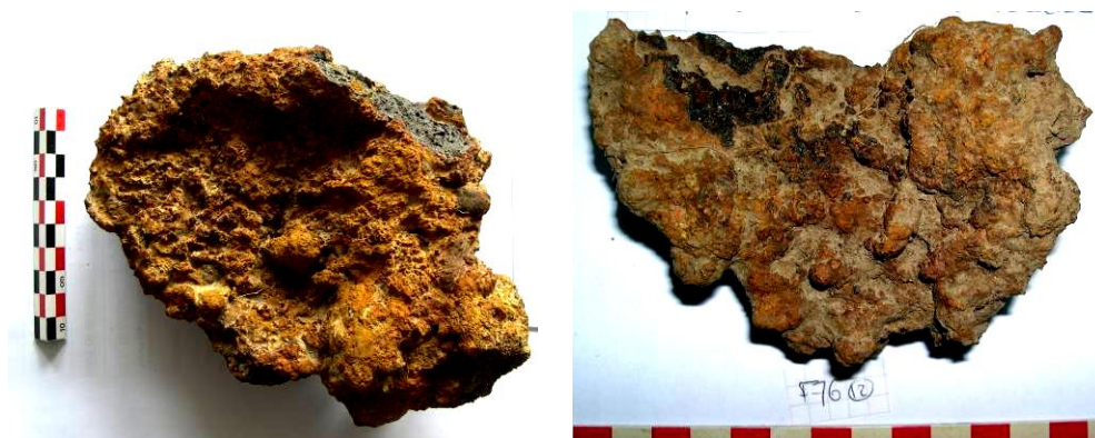
Figure 29 : Scories plano-convexes de forge
